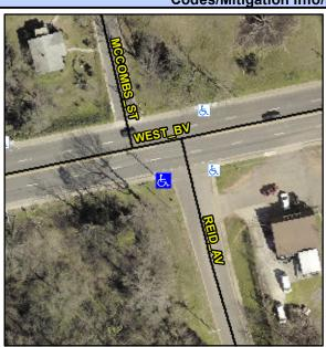
**REID AV** Street 1 Name Stop Condition-Street 2 StopSign Street 2 Name **WEST BV** Stop Condition-Street 1 None Possible Solutions: Remove & Replace Curb Ramp With **Two New Directional Ramps or** Equivalent. Surveyor Notes: N/A PROW/ADA: Not Found, R304.5.1, R304.5.3
