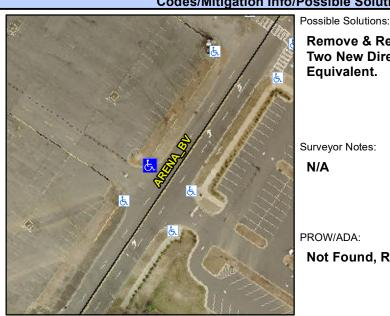
**ENTRANCE** Street 1 Name Stop Condition-Street 2 None **ARENA BV** Street 2 Name Stop Condition-Street 1 None Remove & Replace Curb Ramp With Two New Directional Ramps or Equivalent.
