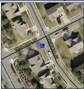
Street 1 Name Stop Condition-Street 1 Street 2 Name Stop Condition-Street 2 **BRECKFIELD CT** StopSign TRAILMOOR RD Possible Solutions: Remove & Replace Curb Ramp With Two New Directional Ramps or Equivalent. Surveyor Notes: N/A PROW/ADA: R304.5.1, R304.5.3
