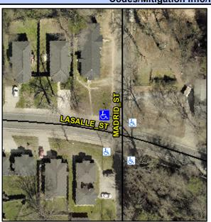
Street 1 Name Stop Condition-Street 2 Street 2 Name Stop Condition-Street 1 LASALLE ST None **MADRID ST** StopSign Possible Solutions: Remove & Replace Curb Ramp With Two New Directional Ramps or Equivalent. Surveyor Notes: N/A PROW/ADA: Not Found, R304.5.1, R304.2.2, R304.5.3
