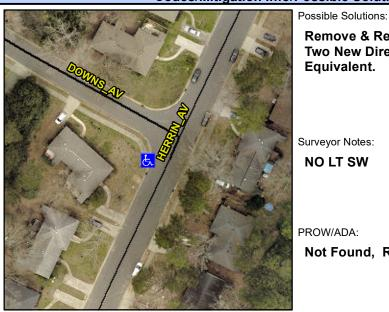
**HERRIN AV** Street 1 Name Stop Condition-Street 1 None Street 2 Name N/A Stop Condition-Street 2 N/A Remove & Replace Curb Ramp With **Two New Directional Ramps or** Equivalent.
