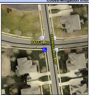
**SPRINGS MILL RD** Street 1 Name Stop Condition-Street 2 None **RAFFIA RD** Street 2 Name Stop Condition-Street 1 StopSign Possible Solutions: Remove & Replace Curb Ramp With Two New Directional Ramps or Equivalent. Surveyor Notes: N/A PROW/ADA: R304.5.1
