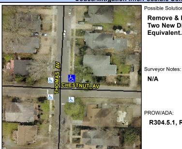
**THOMAS AV** Street 1 Name Stop Condition-Street 2 StopSign Street 2 Name **CHESTNUT AV** Stop Condition-Street 1 StopSign Possible Solutions: Remove & Replace Curb Ramp With Two New Directional Ramps or Equivalent.
