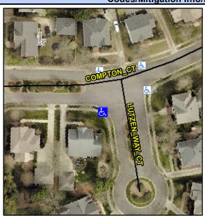
**LUTHERS ROCK CT** Street 1 Name Stop Condition-Street 2 None Street 2 Name **COMPTON CT** Stop Condition-Street 1 None Possible Solutions: Remove & Replace Curb Ramp With **Two New Directional Ramps or** Equivalent. Surveyor Notes: N/A PROW/ADA: Not Found, R304.5.1
