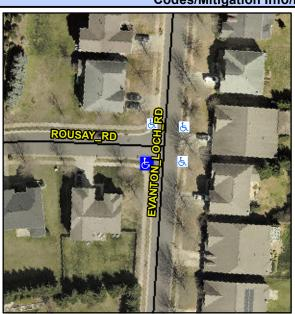
**EVANTON LOCH RD** Street 1 Name Stop Condition-Street 2 None Street 2 Name **ROUSAY RD** Stop Condition-Street 1 StopSign Possible Solutions: **Remove & Replace Curb Ramp With Two New Directional Ramps or** Equivalent. Surveyor Notes: N/A PROW/ADA: R304.5.1, R304.2.2
