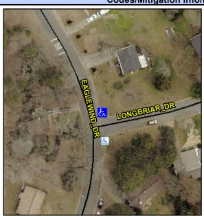
Street 1 Name Stop Condition-Street 2 Street 2 Name Stop Condition-Street 1 **EAGLEWIND DR** None **LONGBRIAR DR** StopSign Possible Solutions: Remove & Replace Curb Ramp With Two New Directional Ramps or Equivalent. Surveyor Notes: N/A PROW/ADA: Not Found, R304.2.2, R304.5.3
