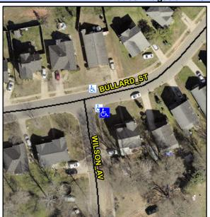
Street 1 Name None Stop Condition-Street 1 **BULLARD ST** Street 2 Name N/A Stop Condition-Street 2 N/A Possible Solutions: Remove & Replace Entire Ramp. Surveyor Notes: **RT RP < 5%** PROW/ADA: Not Found, R304.5.1, R304.5.1, R304.2.2, R304.5.3
