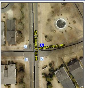
Street 1 Name Stop Condition-Street 2 Street 2 Name Stop Condition-Street 1 WADE ARDREY RD None WHEATFIELD RD StopSign Possible Solutions: **Remove & Replace Curb Ramp With Two New Directional Ramps or** Equivalent. Surveyor Notes: N/A PROW/ADA: R304.5.1, R304.2.2, R304.5.3
