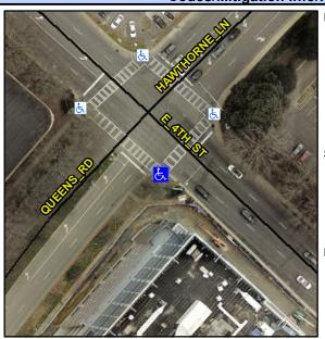
Street 1 Name E 4TH ST Stop Condition-Street 1 Signal Street 2 Name **HAWTHORNE LN** Stop Condition-Street 2 Signal Possible Solutions: Remove & Replace Curb Ramp With Two New Directional Ramps or Equivalent. Surveyor Notes: N/A PROW/ADA: Not Found, R304.5.1, R304.5.3
