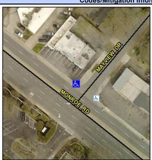
**MAYVIEW DR** Street 1 Name Stop Condition-Street 1 StopSign Street 2 Name N/A Stop Condition-Street 2 N/A Remove & Replace Curb Ramp With **Two New Directional Ramps or** Equivalent.
