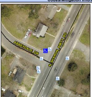
**ABBEYDALE DR** Street 1 Name Stop Condition-Street 2 StopSign Street 2 Name N/A Stop Condition-Street 1 N/A Possible Solutions: Remove & Replace Entire Ramp. Surveyor Notes: N/A PROW/ADA: Not Found, R304.5.1, R304.2.2
