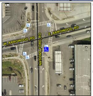
**NATIONS FORD RD** Street 1 Name Stop Condition-Street 1 Signal Street 2 Name N/A Stop Condition-Street 2 N/A Possible Solutions: Remove & Replace Curb Ramp With Two New Directional Ramps or Equivalent. Surveyor Notes: N/A PROW/ADA: R304.5.3
