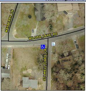
STILLWELL OAKS CR Street 1 Name Stop Condition-Street 1 StopSign N/A Street 2 Name Stop Condition-Street 2 N/A Possible Solutions: Remove & Replace Curb Ramp With Two New Directional Ramps or Equivalent. Surveyor Notes: N/A PROW/ADA: Not Found, R304.5.1, R304.5.3
