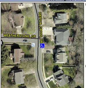
**HATTON CROSS DR** Street 1 Name Stop Condition-Street 1 None Street 2 Name N/A Stop Condition-Street 2 N/A Possible Solutions: Remove & Replace Curb Ramp With **Two New Directional Ramps or** Equivalent. Surveyor Notes: **CURB LIP 2.0** PROW/ADA: Not Found, R304.5.3, R305
