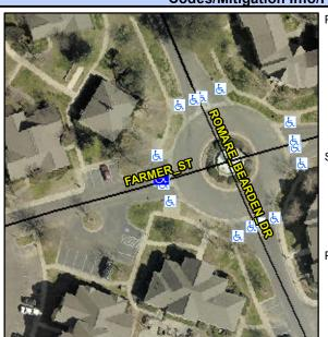
**FARMER ST** Street 1 Name Stop Condition-Street 2 None Street 2 Name N/A Stop Condition-Street 1 N/A Possible Solutions: Remove & Replace Entire Ramp. Surveyor Notes: N/A PROW/ADA: Not Found, R304.5.3, R304.2.1, R304.2.2-Perp, R304.3.2-Para, R305.1.4, R305.2
