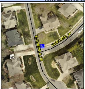
Street 1 Name Stop Condition-Street 2 Street 2 Name Stop Condition-Street 1 **BLOOMFIELD DR** None **ROSELAND AV** StopSign Possible Solutions: Remove & Replace Curb Ramp With Two New Directional Ramps or Equivalent. Surveyor Notes: N/A PROW/ADA: Not Found, R304.5.3
