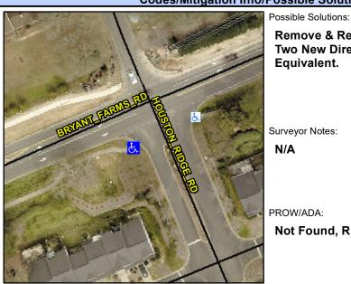
Street 1 Name Stop Condition-Street 2 Street 2 Name Stop Condition-Street 1 **HOUSTON RIDGE RD** StopSign **BRYANT FARMS RD**  Remove & Replace Curb Ramp With Two New Directional Ramps or Equivalent.
