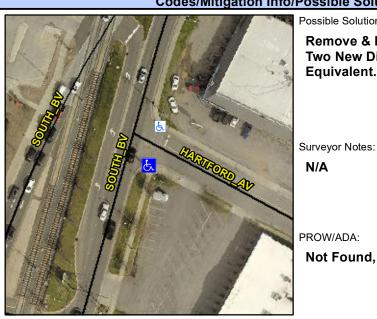
Street 1 Name Stop Condition-Street 2 Street 2 Name Stop Condition-Street 1 HARTFORD AV StopSign **SOUTH BV** None Possible Solutions: Remove & Replace Curb Ramp With **Two New Directional Ramps or** Equivalent.
