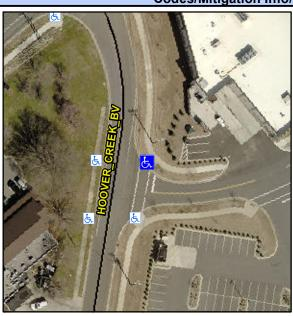
Street 1 Name Stop Condition-Street 2 Street 2 Name Stop Condition-Street 1 **HOOVER CREEK BV** None **ENTRANCE** StopSign Possible Solutions: Remove & Replace Curb Ramp With **Two New Directional Ramps or** Equivalent. Surveyor Notes: N/A PROW/ADA: Not Found, R304.5.1
