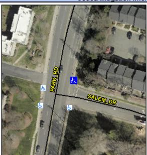
Street 1 Name **PARK RD** Stop Condition-Street 2 None **SALEM DR** Street 2 Name Stop Condition-Street 1 StopSign Possible Solutions: Remove & Replace Curb Ramp With Two New Directional Ramps or Equivalent. Restripe Crosswalk. Surveyor Notes: N/A PROW/ADA: Not Found, R304.2.2, R304.5.3
