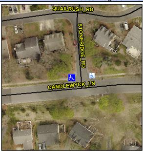
**CANDLEWYCK LN** Street 1 Name Stop Condition-Street 2 None STONERIDGE RD Street 2 Name Stop Condition-Street 1 StopSign Possible Solutions: Remove & Replace Curb Ramp With Two New Directional Ramps or Equivalent. Surveyor Notes: N/A PROW/ADA: R304.2.2, R304.5.3
