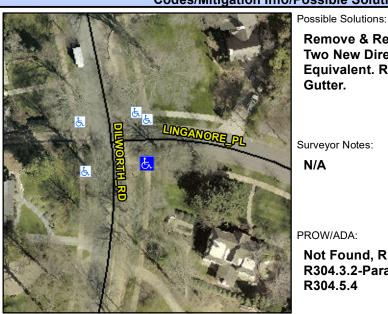
Street 1 Name Stop Condition-Street 2 Street 2 Name Stop Condition-Street 1 LINGANORE PL StopSign **DILWORTH RD** None Remove & Replace Curb Ramp With Two New Directional Ramps or Equivalent. Remove & Replace Gutter.
