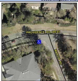
**MARVIN RD** Street 1 Name Stop Condition-Street 1 StopSign PROVIDENCE RD WEST Street 2 Name Stop Condition-Street 2 None Possible Solutions: Remove & Replace Curb Ramp With Two New Directional Ramps or Equivalent. Surveyor Notes: N/A PROW/ADA: Not Found, R304.5.1
