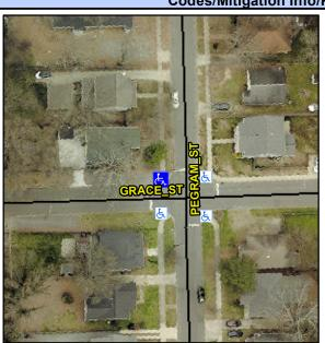
**GRACE ST** Street 1 Name Stop Condition-Street 2 StopSign **PEGRAM ST** Street 2 Name Stop Condition-Street 1 StopSign Possible Solutions: Remove & Replace Curb Ramp With **Two New Directional Ramps or** Equivalent. Surveyor Notes: N/A PROW/ADA: Not Found, R304.5.3, R305.1.4, R305.2, R302.7, R302.7.2
