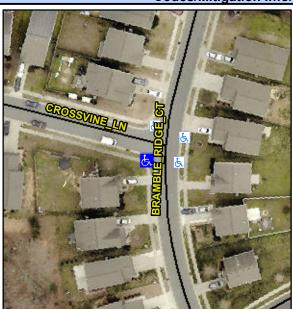
Street 1 Name Stop Condition-Street 2 Street 2 Name Stop Condition-Street 1 **BRAMBLE RIDGE CT** None **CROSSVINE LN** StopSign Possible Solutions: **Remove & Replace Curb Ramp With Two New Directional Ramps or** Equivalent. Surveyor Notes: N/A PROW/ADA: Not Found, R305.2, R302.7.2
