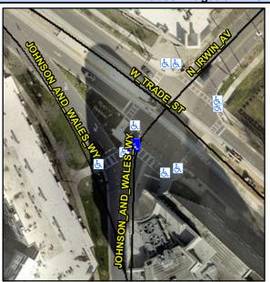
**JOHNSON AND WALES WY** Street 1 Name Stop Condition-Street 1 Signal N/A Street 2 Name Stop Condition-Street 2 N/A Possible Solutions: Remove & Replace Landing. Surveyor Notes: **LOCATED ON ISLAND** PROW/ADA: R304.2.2-Perp, R304.3.2-Para
