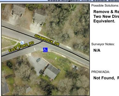
**EAST FORD RD** Street 1 Name Stop Condition-Street 1 StopSign N/A Street 2 Name Stop Condition-Street 2 N/A Remove & Replace Curb Ramp With Two New Directional Ramps or Equivalent.
