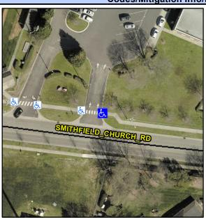
**ENTRANCE** Street 1 Name Stop Condition-Street 1 StopSign N/A Street 2 Name Stop Condition-Street 2 N/A Possible Solutions: Compliance Description N/A Remove & Replace Curb Ramp With Two New Directional Ramps or Equivalent. Surveyor Notes: N/A PROW/ADA: Not Found, R304.5.1
