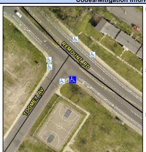
REMOUNT RD Street 1 Name Stop Condition-Street 2 None N/A Street 2 Name Stop Condition-Street 1 N/A Possible Solutions: Remove & Replace Entire Ramp. Surveyor Notes: N/A PROW/ADA: Not Found, R304.2.2, R304.5.3
