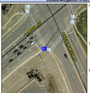
Street 1 Name **S TRYON ST** Stop Condition-Street 2 Signal Street 2 Name N/A Stop Condition-Street 1 N/A Possible Solutions: Remove & Replace Entire Ramp. Surveyor Notes: N/A PROW/ADA: R304.5.1, R304.2.2
