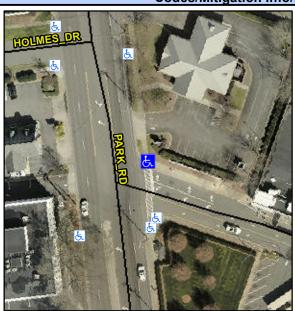
PARK RD Street 1 Name Stop Condition-Street 2 None PARKING SHOPPING CENTER DR Street 2 Name Stop Condition-Street 1 StopSign Possible Solutions: Remove & Replace Curb Ramp With Two New Directional Ramps or Equivalent. Surveyor Notes: N/A PROW/ADA: Not Found, R304.5.1
