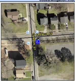
**FRENCH ST** Street 1 Name Stop Condition-Street 2 StopSign **CAMPUS ST** Street 2 Name Stop Condition-Street 1 None Possible Solutions: Remove & Replace Curb Ramp With **Two New Directional Ramps or** Equivalent. Surveyor Notes: N/A PROW/ADA: Not Found, R304.2.2
