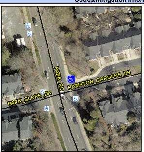
PARK RD Street 1 Name Stop Condition-Street 2 Street 2 Name **HAMPTON GARDENS LN** Stop Condition-Street 1 StopSign Possible Solutions: Remove & Replace Curb Ramp With Two New Directional Ramps or Equivalent. Surveyor Notes: N/A PROW/ADA: Not Found, R304.5.1, R304.2.2, R304.5.3
