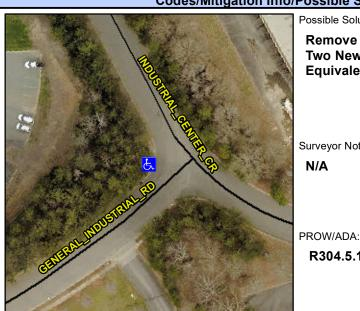
Street 1 Name Stop Condition-Street 2 Street 2 Name Stop Condition-Street 1 **GENERAL INDUSTRIAL RD** StopSign **INDUSTRIAL CENTER CR**  Possible Solutions: Remove & Replace Curb Ramp With Two New Directional Ramps or Equivalent. Surveyor Notes: N/A
