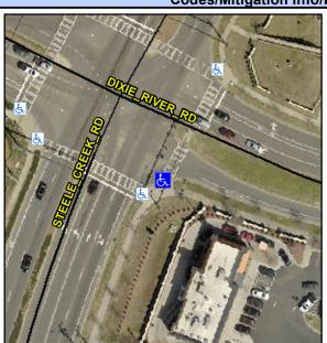
STEELE CREEK RD Street 1 Name Stop Condition-Street 2 Signal Street 2 Name N/A Stop Condition-Street 1 N/A Possible Solutions: Remove & Replace Entire Ramp. Surveyor Notes: N/A PROW/ADA: R304.5.1, R304.2.2, R304.5.3
