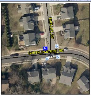
**GREEN PASTURE RD** Street 1 Name Stop Condition-Street 2 **SHELLEY AV** Street 2 Name Stop Condition-Street 1 StopSign Possible Solutions: Remove & Replace Curb Ramp With Two New Directional Ramps or Equivalent.
