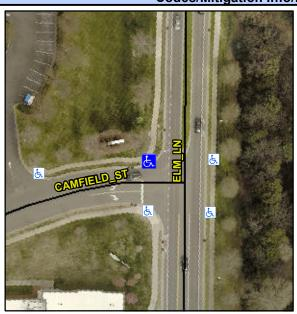
**CAMFIELD ST** Street 1 Name Stop Condition-Street 2 StopSign **ELM LN** Street 2 Name Stop Condition-Street 1 None Possible Solutions: Remove & Replace Curb Ramp With Two New Directional Ramps or Equivalent. Surveyor Notes: N/A PROW/ADA: Not Found, R304.5.1, R304.2.2, R304.5.3
