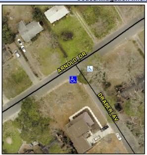
**DRAPER AV** Street 1 Name Stop Condition-Street 2 StopSign Street 2 Name N/A Stop Condition-Street 1 N/A Possible Solutions: Remove & Replace Entire Ramp. Surveyor Notes: N/A PROW/ADA: Not Found, R304.2.1, R304.2.2-Perp, R304.3.2-Para, R304.5.3, R305, R302.7.2
