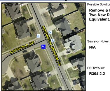
**HUNTINGTON MEADOW LN** Street 1 Name Stop Condition-Street 2 None Street 2 Name **SOUTHFIELD DR** Stop Condition-Street 1 StopSign Possible Solutions: Remove & Replace Curb Ramp With **Two New Directional Ramps or** Equivalent.
