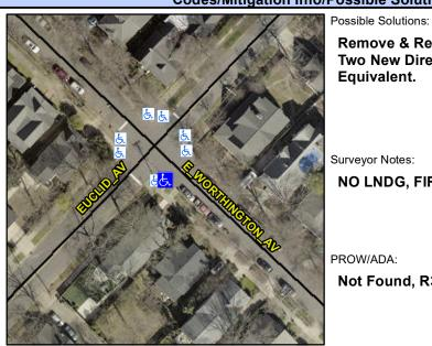
**E WORTHINGTON AV** Street 1 Name Stop Condition-Street 1 StopSign Street 2 Name N/A Stop Condition-Street 2 N/A Remove & Replace Curb Ramp With Two New Directional Ramps or Equivalent.
