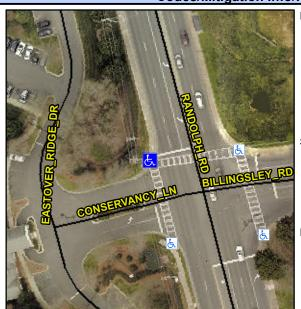
Street 1 Name Stop Condition-Street 2 Street 2 Name Stop Condition-Street 1 **CONSERVANCY LN** Signal **RANDOLPH RD** Signal Possible Solutions: Remove & Replace Curb Ramp With **Two New Directional Ramps or Equivalent. Restripe Crosswalk.** Surveyor Notes: N/A PROW/ADA: R304.5.1
