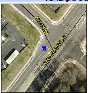
Street 1 Name **BAUCOM RD** Stop Condition-Street 2 StopSign Street 2 Name N/A Stop Condition-Street 1 N/A Possible Solutions: Remove & Replace Entire Ramp. Surveyor Notes: N/A PROW/ADA: Not Found, R304.5.1, R304.5.3
