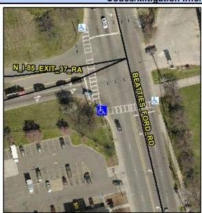
Street 1 Name **BEATTIES FORD RD** Stop Condition-Street 2 Signal Street 2 Name N I-85 EXIT 37 RA Stop Condition-Street 1 Signal Possible Solutions: **Remove & Replace Curb Ramp With Two New Directional Ramps or** Equivalent. Surveyor Notes: N/A PROW/ADA: Not Found, R304.2.2
