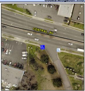
Street 1 Name None Stop Condition-Street 1 **ENTRANCE** Street 2 Name None Stop Condition-Street 2 **CENTRAL AV**  Possible Solutions: Remove & Replace Curb Ramp With Two New Directional Ramps or Equivalent. Surveyor Notes: **MEDIAN ACROSS CENTRAL AV** PROW/ADA: Not Found, R304.5.1, R304.5.3, R304.3.2
