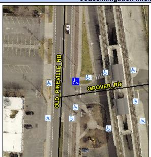
**OLD PINEVILLE RD** Street 1 Name Stop Condition-Street 2 None **GROVER RD** Street 2 Name Stop Condition-Street 1 StopSign Possible Solutions: Remove & Replace Curb Ramp With **Two New Directional Ramps or** Equivalent. Surveyor Notes: N/A
