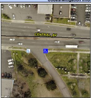
Street 1 Name Stop Condition-Street 2 Street 2 Name Stop Condition-Street 1 **CENTRAL AV** None **ENTRANCE** None Possible Solutions: Remove & Replace Curb Ramp With **Two New Directional Ramps or** Equivalent. Surveyor Notes: N/A PROW/ADA: Not Found, R304.5.1, R304.5.3
